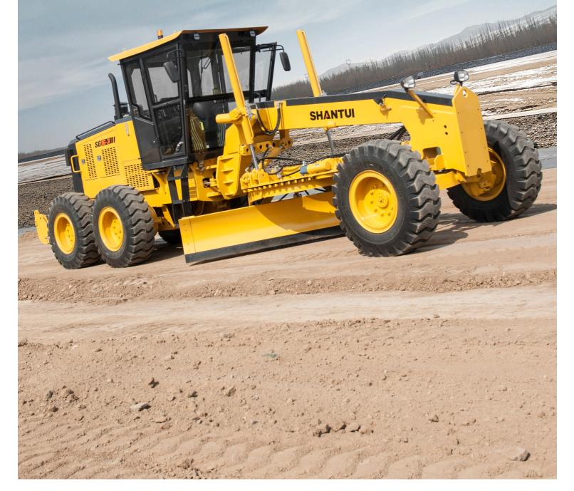
Engine Model: Gross Power: Operating Weight: Cummins 6BTAA5.9-C160 118kW @ 2200rpm 15,100kg We Level Subgrade Fast and Flat easy operation and maintenance
