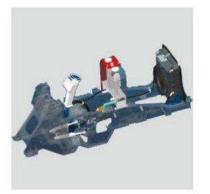
Load sensing steering maximizes machine performance by directing power through the steering system only when needed. When the machine is not steering, more engine power is available to generate rimpull, breakout and lift forces.
